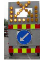
Warning panel with: • Signal 1098 "Flashing yellow light signal" • Signal 1100 "Flashing light arrows" • Sign 930 "Closure markers" and • Sign 404.2 "Mandatory driving lane"
