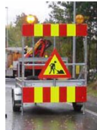
Warning panel with: • Signal 1098 "Flashing yellow light signal" • Sign 930 "Closure markers" and • Sign 110 "Roadworks"
